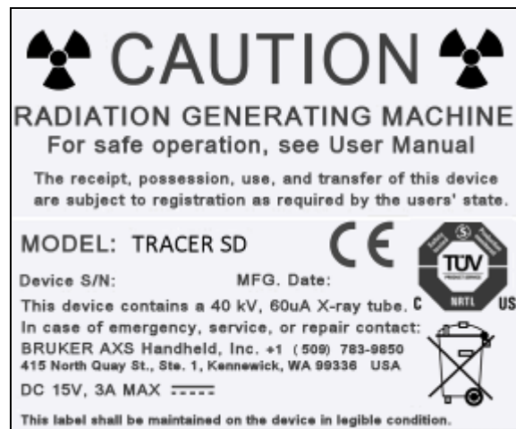
Example of Manufacturers' regulatory plate located underneath analyzer.
