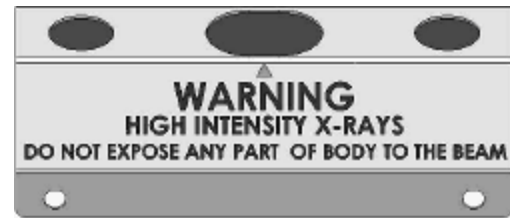
WARNING Sign located on clip-on window protector.
